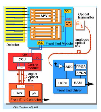
Data acquisition electronics of our module testing setup are similar to the electronis that will be used in the CMS experiment.
