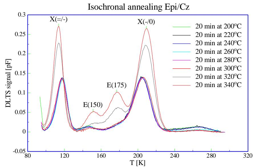
The X-level is also generated in STFZ material, ***but*** after annealing out of  $V_2$
