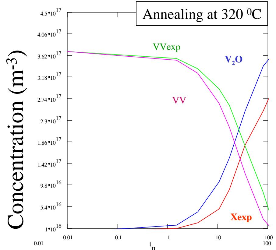
The impurity which forms the X center via VV migration should be in a much smaller concentration than that of oxygen interstitial
