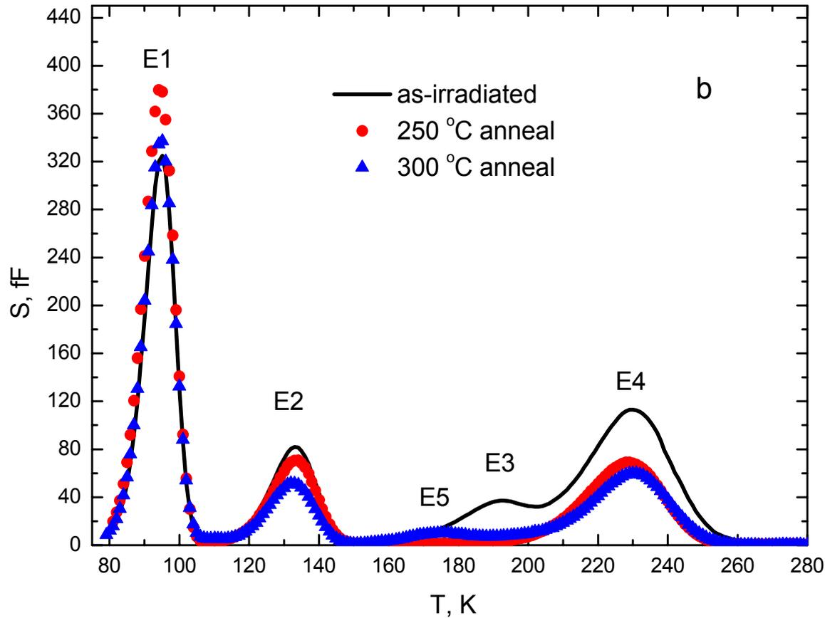
Fig.1b. Development of DLTS spectra for standard FZ diodes (W-sample) after electron irradiation at room temperature and upon 30-min isochronal annealing with temperature increments of 50 °C. Dose of irradiation was  $2 \times 10^{12} \text{ cm}^{-2}$  ( $E_e=6 \text{ MeV}$ ). Measurement settings were  $e_n = 190 \text{ s}^{-1}$ , bias  $-5 \rightarrow 0 \text{ V}$ , and pulse duration = 10 ms
