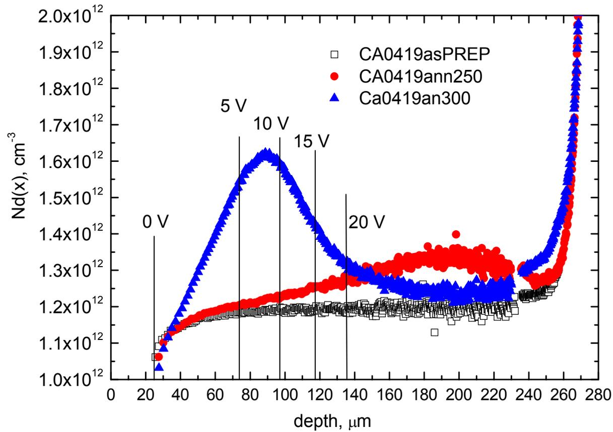
Fig.9. Carrier depth profile for a CA sample determined from C-V characteristics. Vertical lines mark inverse voltage which is necessary to obtain indicated width of depletion region.
