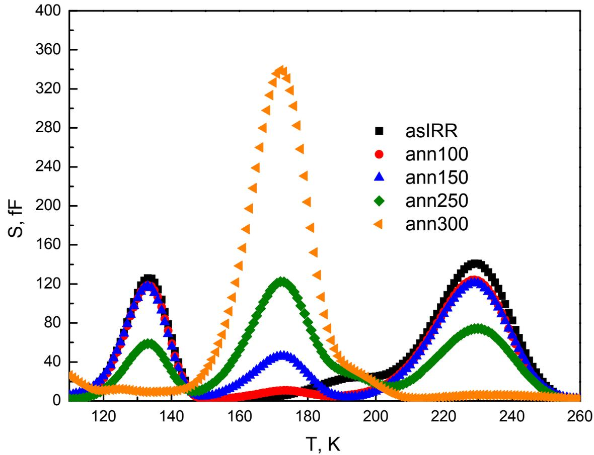
Fig. 7. Development of DLTS spectra for hydrogenated standard FZ diode(CA-sample) after irradiation with 3.5 MeV electrons at room temperature and upon 30-min isochronal annealing with temperature increments of 50 °C. Dose of irradiation was  $3 \times 10^{12} \text{ cm}^{-2}$ . Measurement settings were  $e_n = 190 \text{ s}^{-1}$ , bias  $-5 \rightarrow -0 \text{ V}$ , and pulse duration 10 ms.
