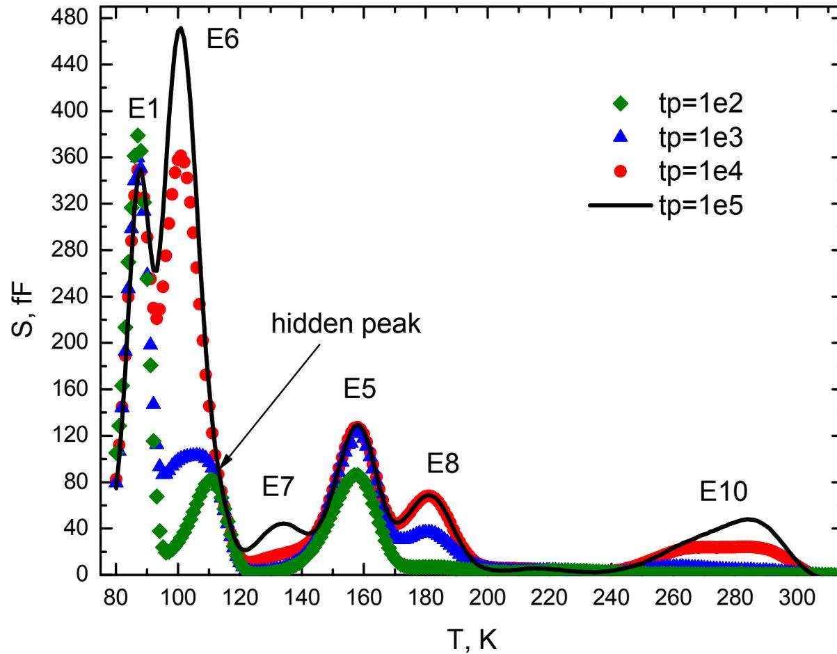
Fig.3. DLTS spectra for standard FZ diode (CA-sample) after isochronal annealing at temperature 350 °C. Measurement settings were  $e_n = 19 \text{ s}^{-1}$ , bias  $-5 \rightarrow 0 \text{ V}$ , and pulse duration ( $t_p$ ): 0.1 ms, 1 ms, 10 ms, 100 ms.
