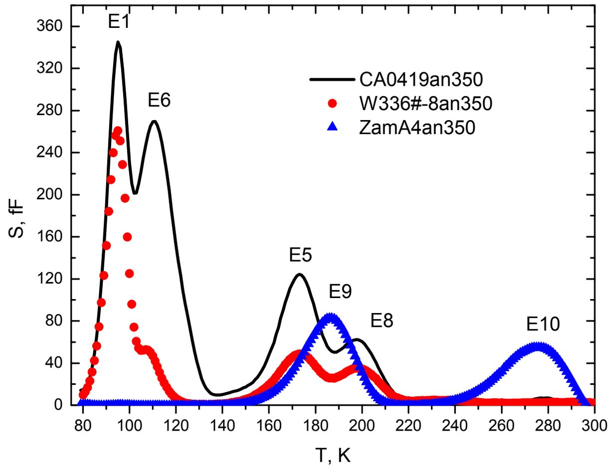
Fig. 2. DLTS spectra for different diodes made of standard FZ silicon after isochronal annealing at temperature 350 °C during 30 min. Measurement settings were  $e_n = 190 \text{ s}^{-1}$ , bias  $-5 \rightarrow 0 \text{ V}$ , and pulse duration ( $t_p$ ) - 10 ms
