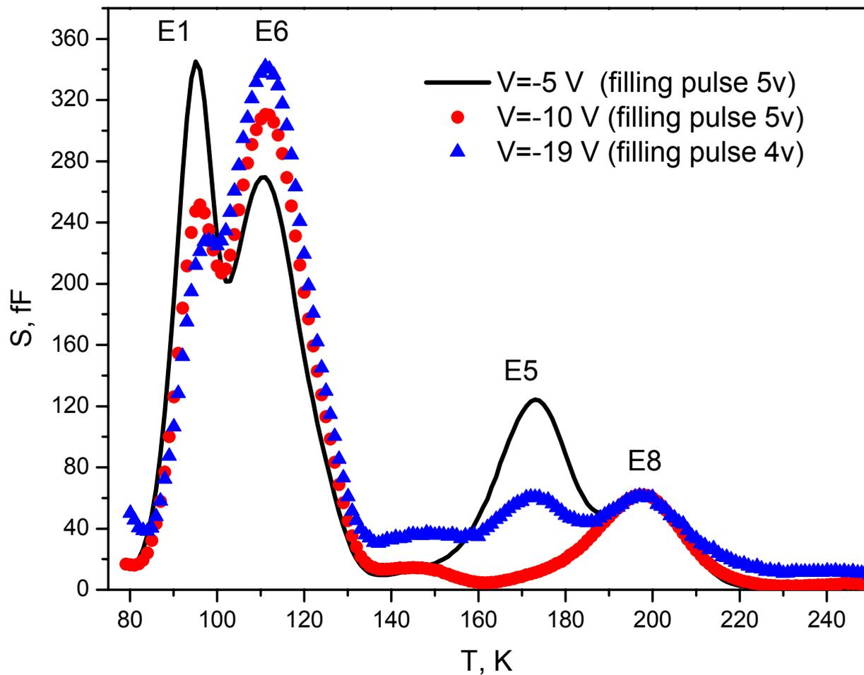
Fig.5. DLTS spectra for standard FZ diode (CA-sample) after irradiation with 3.5 MeV electrons at room temperature and upon 30-min annealing at 350 °C.. Dose of irradiation was  $3 \times 10^{12}$  cm<sup>-2</sup>. Measurement settings were: rate window of 190 s<sup>-1</sup>, pulse duration of 10 ms, bias: a) -5 → 0 V, b) -10 → -5 V and c) -19 → -15 V. The peak amplitudes are normalized assuming constant concentration of E8 trap.
