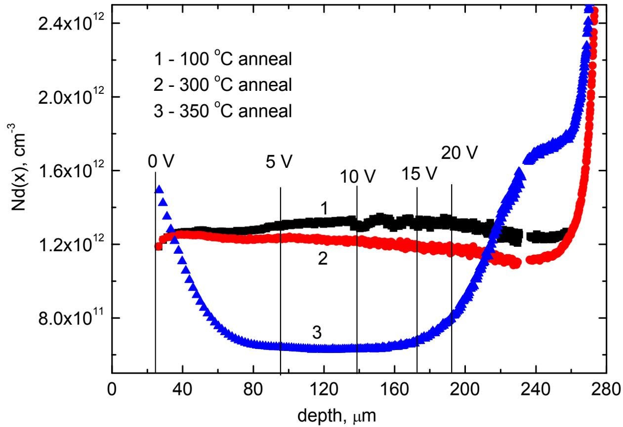
Fig 6. Carrier depth profile for a CA sample determined from C-V characteristics.
