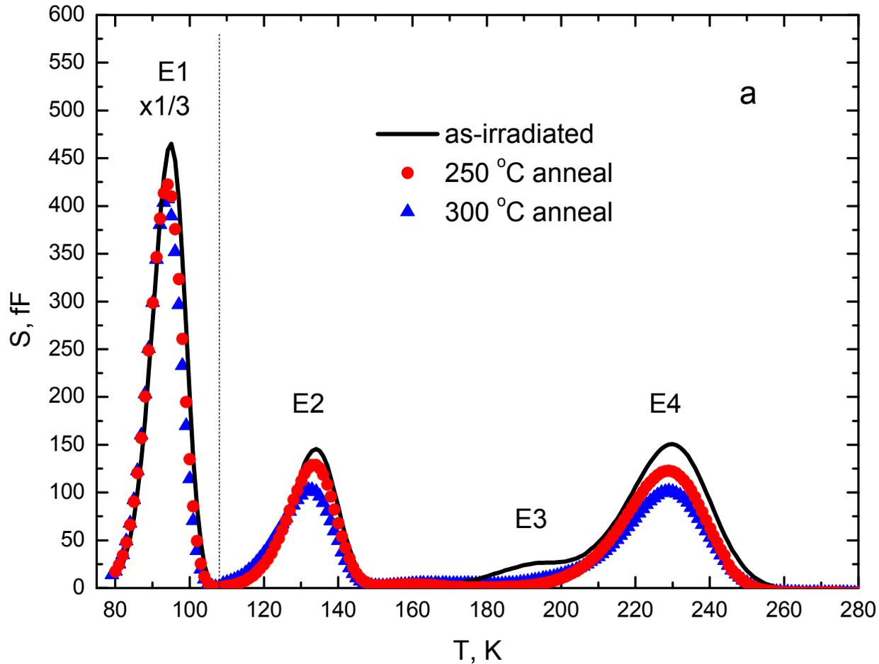
Fig.1a. Development of DLTS spectra for standard FZ diodes (CA-sample) after electron irradiation at room temperature and upon 30-min isochronal annealing with temperature increments of 50 °C. Dose of irradiation was  $2 \times 10^{12} \text{ cm}^{-2}$  ( $E_e = 3.5 \text{ MeV}$ ). Measurement settings were  $e_n = 190 \text{ s}^{-1}$ , bias  $-5 \rightarrow 0 \text{ V}$ , and pulse duration = 10 ms.
