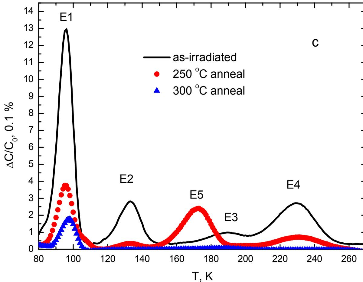
Fig.1c. Development of DLTS spectra for standard FZ diodes (ZA-sample) after electron irradiation at room temperature and upon 30-min isochronal annealing with temperature increments of 50 °C. Dose of irradiation was  $1 \times 10^{12} \text{ cm}^{-2}$  ( $E_e=6 \text{ MeV}$ ). Measurement settings were  $e_n = 190 \text{ s}^{-1}$ , bias  $-5 \rightarrow 0 \text{ V}$ , and pulse duration = 10 ms
