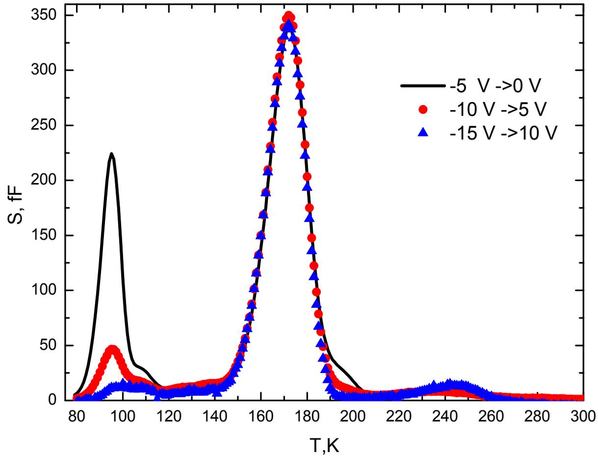
Fig.8. DLTS spectra for hydrogenated standard FZ diode(CA-sample) after irradiation with 3.5 MeV electrons at room temperature and upon 30-min annealing at 300 °C. Dose of irradiation was  $3 \times 10^{12} \text{ cm}^{-2}$ . Measurement settings were  $e_n = 190 \text{ s}^{-1}$ , pulse duration 10 ms bias: a) -5 → 0 V, b) -10 → -5 V, b) -15 → -10 V. All spectra normalized the E5 peak (VOH) amplitude.
