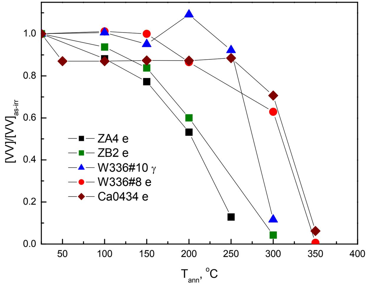
Fig.4. Annealing behavior of divacancy (trap E2) in different diodes irradiated with electrons or gamma-rays (W336 diodes).
