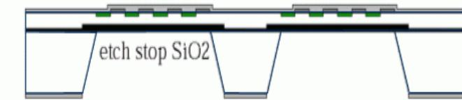
d) anisotropic deep etching opens "windows" in handle wafer
