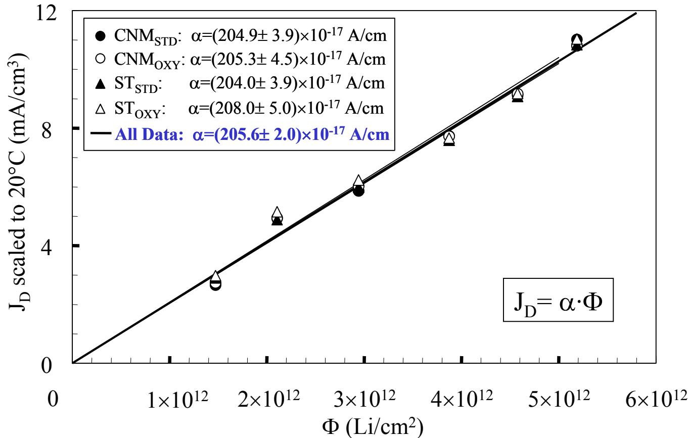
Experimental hardness factor:  $H_{EXP} = \alpha(58 \text{ MeV Li}) / \alpha(1 \text{ MeV neutrons}) = 45.08$
