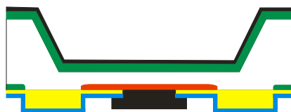
Cross section of a thinned silicon detector
