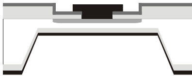
Cross section of a thinned silicon detector by IRST-Trento
