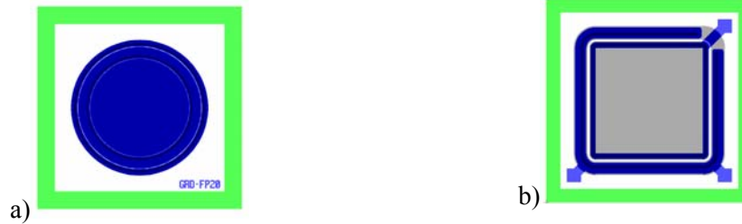
Figure 54: Layout of thinned diodes available on the processed wafers. a) Circular diode having an area of 2.27 \text{ mm}^2 and double guard ring; b) Square diodes of various area: 0.75 , 1.9 , 3.5 , 11.35 \text{ mm}^2 .
