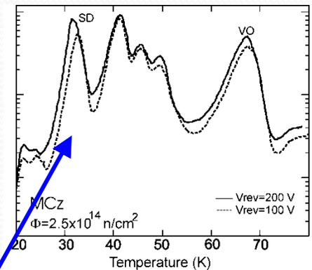
MCz n-type 26 MeV p irradiated,  $\Phi=4 \times 10^{14} \text{ cm}^{-2}$
