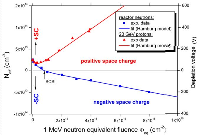
Epitaxial silicon (EPI-DO, 72 $\mu$ m, 170 $\Omega$ cm, diodes) irradiated with **23 GeV protons**
