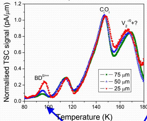
Epi 50 $\mu\text{m}$  23 GeV p irradiated,  $\Phi=4 \times 10^{14} \text{ cm}^{-2}$
