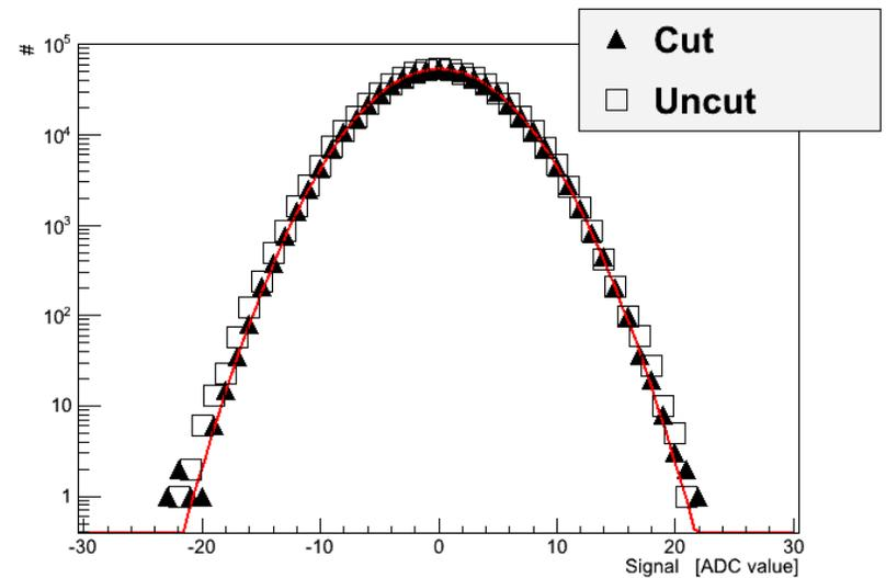
The signal from a beta source before and after cutting is the same within 4%. The noise on all strips, including the one adjacent to the slim edge, is not changed by the cut.
