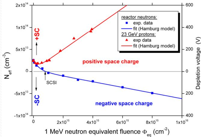
Epitaxial silicon (*EPI-DO, 72 $\mu\text{m}$ , 170 $\Omega\text{cm}$ , diodes*) irradiated with reactor neutrons
