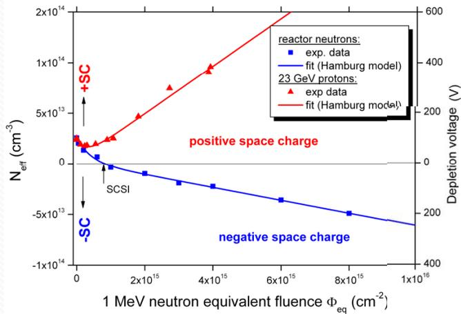
Epitaxial silicon (EPI-DO, 72 $\mu\text{m}$ , 170 $\Omega\text{cm}$ , diodes) irradiated with **23 GeV protons**
