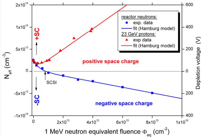
Epitaxial silicon (*EPI-DO, 72 $\mu$ m, 170 $\Omega$ cm, diodes*) irradiated with reactor neutrons
