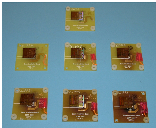
Figure 2: Test Structure Arrays on PCBs after Irradiations to Fluences of 0, 4 \times 10^{13} , 1 \times 10^{14} , 3.5 \times 10^{14} , 1 \times 10^{15} , 3.6 \times 10^{15} and 1 \times 10^{16} .
